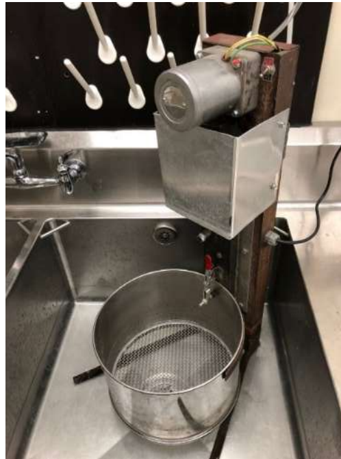
The wet sieving unit developed by CVAS. The unit moves the sieve up and down in water approximately 60 times per minute to wash particles through the 4.75 mm sieve aperture.
